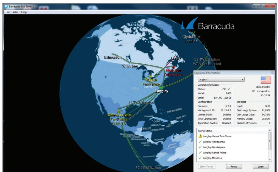
*Barracuda NG Earth is a graphical real-time 3D network monitoring utility that provides a status overview of all VPN site-to-site tunnels.*
