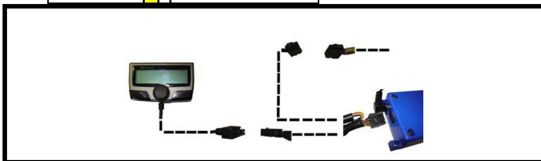
Connect the LCD harness to the adapter.
