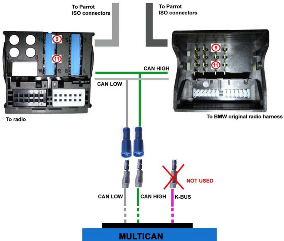
**Connect the white wire corresponding to CAN Low to pin 9.
