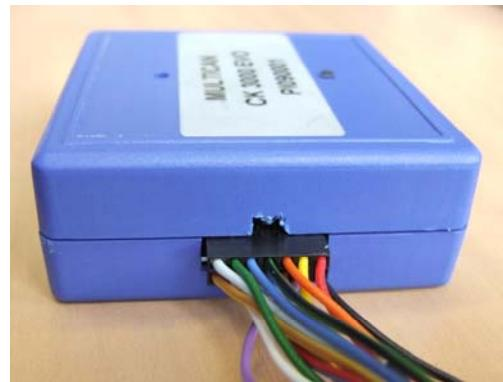
Connect the power cable of the MULTICAN interface to the 14-way connector of the MULTICAN interface.
